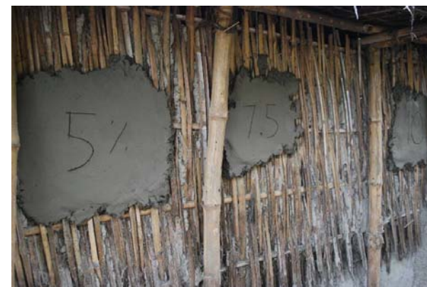
Testing cement stabilised mud
